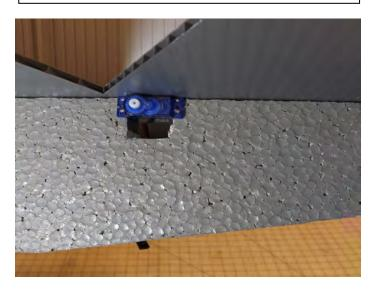
Install the outboard servo into the mounting hole and glue in place, stacked on top of inboard servo. We recommend 9 gram sub micro or similar type servo.
