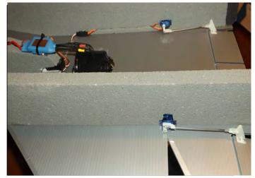
Two more servos are placed on the inboard side of the nacelles opposite and below outboard servos as seen on page 15 and 16.
