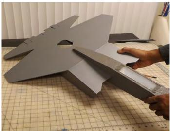
Apply 5 minute epoxy to both sides of fuselage wing slot. Slide the fuselage onto the wing. Be sure that the fuselage is centered straight and square to wing.
