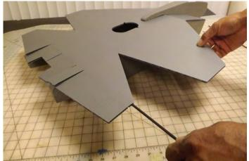
Apply a little 5 minute epoxy to the 30 inch carbon fiber shaft, then insert it in a wing approximately 2nd flute from trailing edge (see photo)
