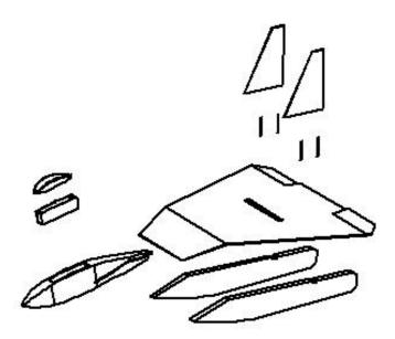
Use this exploded view to help guide you through the assembly of the major components of your Tough Jet.
