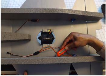
Servo wire exits on inside of nacelle.
