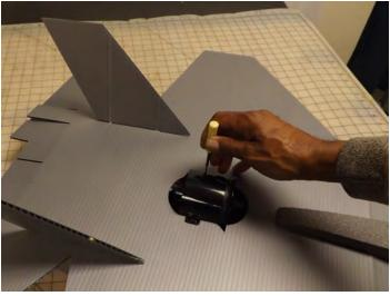
Line up motor straight and square. Mark location and drill holes.
