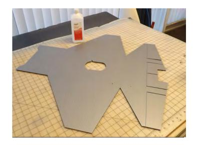
Lay wing on a flat surface, bottom side up. This is the side with the hinge slots and crease.
