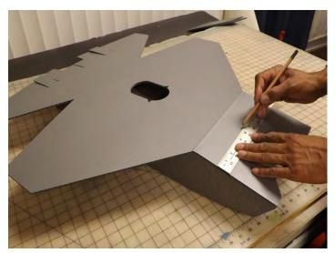
Turn the wing over, measure and mark on the top the center of the wing
