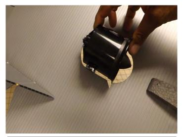
Set your EDF unit in wing with ESC wires facing down **DO NOT** omit intake ring
