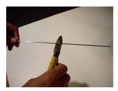
Measure and cut the push rod to fit between the servo arm and control horn.
