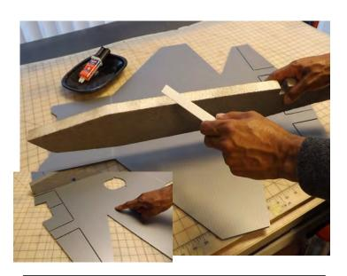
Apply 5 minute epoxy to top of nacelle on flat section only. **Do not** apply epoxy to slanted section at this time. **Do not** let epoxy clog vertical stab dowel holes **see insert photo**
