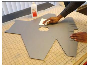
Clean the bottom of the wing with rubbing alcohol before gluing
