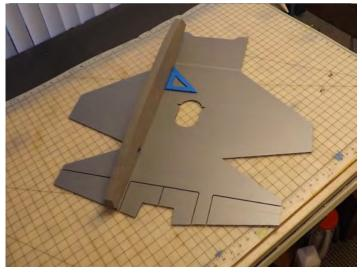
Ensure the nacelle is parallel and 90 degrees to flutes on wing. You have some time to make slight adjustments before epoxy cures but move quickly.
