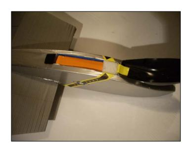
Place the foam filler in front of the battery for flying on non-windy days. You will find if you use the recommended equipment to complete this plane, it will not require any further balancing. Center of Gravity to be 9" to 11 1/4" from leading edge of wing
