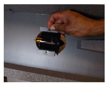
Bolt mount through wing and Coroplast® stiffener don't over tighten bolts.
