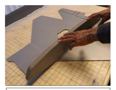
Hold the nacelle in place until the fiveminute epoxy cures, check that nacelle is aligned with leading edge, crease and centered on Vertical stabilizer dowel holes on wing.
