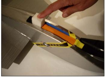
The battery box located on the front of the plane is designed to accept 4-cell lipo 14.8 volt 2200 mah or 2600 mah battery.
