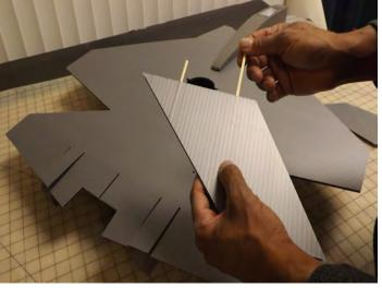
Epoxy 2 dowels into the flutes of each vertical stabilizers. Position the dowels 1" and 4 3/8" from the trailing edge. Leave about 1 ½" of dowel exposed
