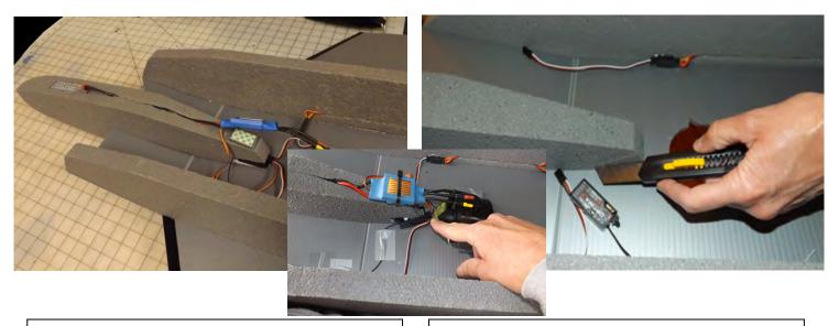
Embed electronic speed control battery wires in slot. Use double sided tape to hold speed control in place.
