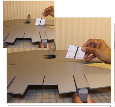
Use alignment tool to open Vertical stabilizer dowel holes to poke hole in foam for dowels press tool flush with top of wing insert sharp dowel into foam.
