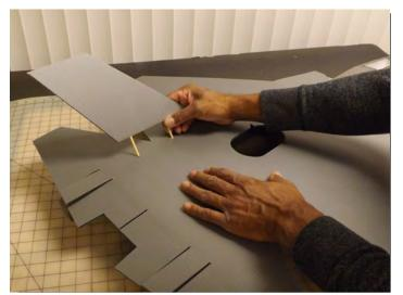
insert stabilizer dowels matching the same angle set by alignment tool it should be a tight fit not needing glue, remaining removable for transporting.
